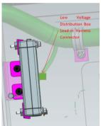
The lead-in harness connector (reserved for the vehicle) of the low-voltage distribution box is located under the auxiliary dashboard, and the detailed position is near the alcohol lock ECU, which can be seen when opening the auxiliary dashboard.
