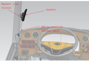
The ECU is concealed and installed below the instrument panel. The ECU harness is connected to the vehicle harness.
