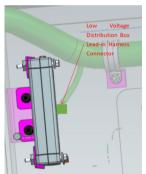
The lead-in harness connector (reserved for the vehicle) of the low-voltage distribution box is located under the auxiliary dashboard, and the detailed position is near the alcohol lock ECU, which can be seen when opening the auxiliary dashboard.
