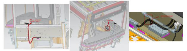
The lead-in harness connector (reserved for the vehicle) of the low-voltage distribution box is located under the auxiliary dashboard, and the detailed position is near the alcohol lock ECU, which can be seen when opening the auxiliary dashboard.
