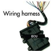
1. Prepare the ECU wire harness by stripping all wires 2 to 4 cm, and apply heat shrink tubing to all wires except the red, black and white wires.
