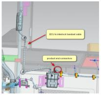
The lead-in harness connector (reserved for the vehicle) of the low-voltage distribution box is located under the auxiliary dashboard, and the detailed position is near the alcohol lock ECU, which can be seen when opening the auxiliary dashboard.
