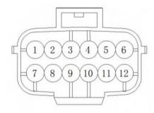
(2) Projection diagram of wire harness end connectors: (Distribution box end harness on vehicle, connect with ECU end connectors)
