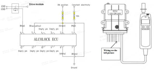
The detailed guide pin definition is shown in the table.
