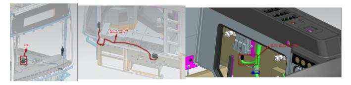
The lead-in harness connector (reserved for the vehicle) of the low-voltage distribution box is located under the auxiliary dashboard, and the detailed position is near the alcohol lock ECU, which can be seen when opening the auxiliary dashboard.
