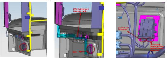
The lead-in harness connector (reserved for the vehicle) of the low-voltage distribution box is located under the auxiliary dashboard, and the detailed position is near the alcohol lock ECU, which can be seen when opening the auxiliary dashboard.
