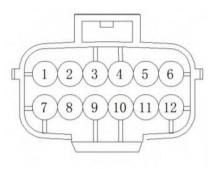
(2) Projection diagram of wire harness end connectors: (Distribution box end harness on vehicle, connect with ECU end connectors)
