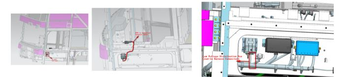
The lead-in harness connector (reserved for the vehicle) of the low-voltage distribution box is located under the auxiliary dashboard, and the detailed position is near the alcohol lock ECU, which can be seen when opening the auxiliary dashboard.
